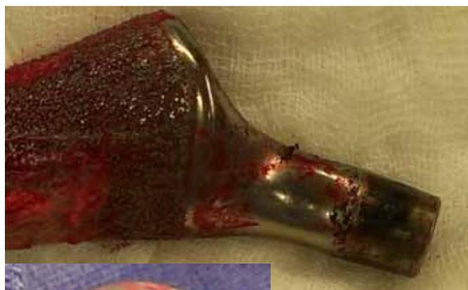
Figure 8: Note the metallic staining and obvious fretting about the trunion.
